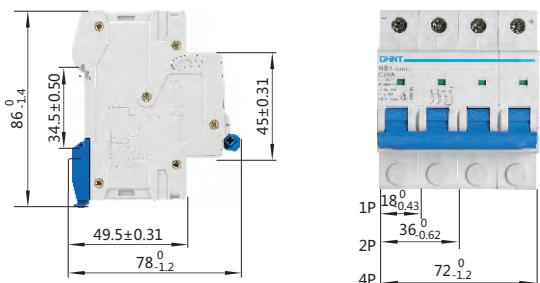
5.6 Wiring: Apply to 25 mm<sup>2</sup> wire connection terminals
