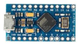
This Pro Micro 5V 16M Mini Leonardo Micro-controller Development Board For Arduino development board has 4 channel 10 bit ADC, 5 PWM pins, 12 DIO, and a hardware serial connection Rx and Tx with Running on 16MHz and 5V.
