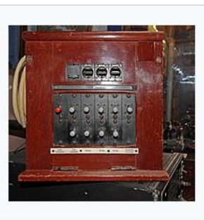
Early 1945 telephone exchange model N935 system featuring cordless operation.
