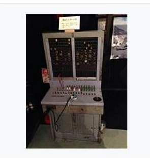
Manual cord telephone exchange exhibited in Ainokura Traditional Industry Museum in Japan.
