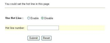
This function supports auto dial for you to set a hot line number. When you set this function the device should not dial any number.
