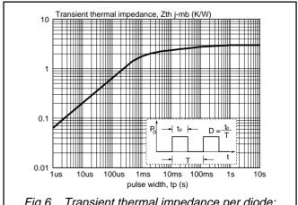
Fig.6. Transient thermal impedance per diode;  $Z_{th j-mb} = f(t_p)$ .
