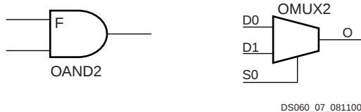
Figure 7: AND and MUX Symbols in Spartan-XL IOB
