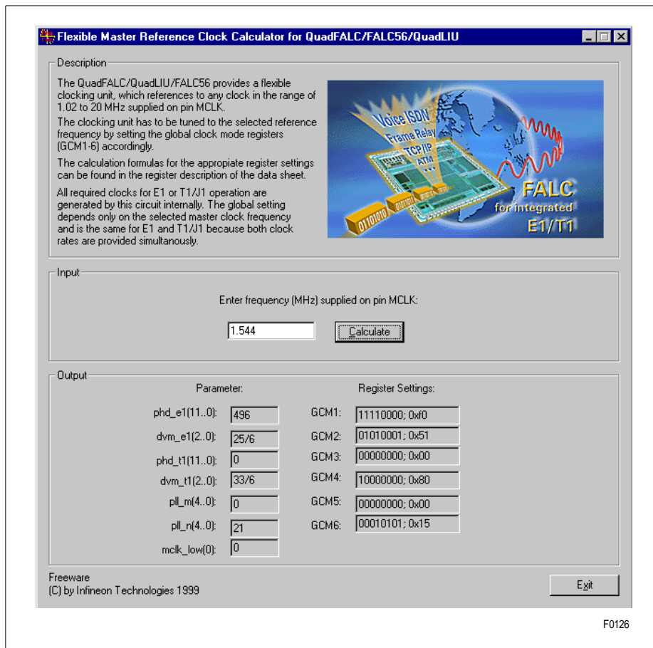
Figure 109 Master Clock Frequency Calculator
