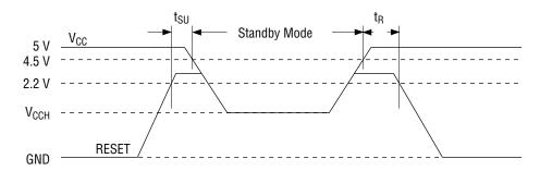
Note: In this case, the C/S register is reset, the port is set into the input mode, and the timer stops.
