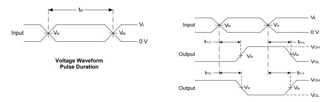
Voltage Waveform Propagation Delay Times Inverting and Non Inverting Outputs
