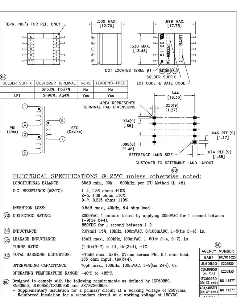
Unless otherwise specified: Tolerances: Angles: ±1' Fractions: ±1/64 Decimals: ±.005[.13] This drawing is dual dimensioned. Dimensions in brackets are in
