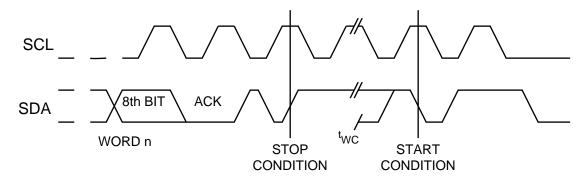
Note: The write cycle time  $t_{wc}$  is the time from a valid stop condition of a write sequence to the end of the internal clear / write cycle.
