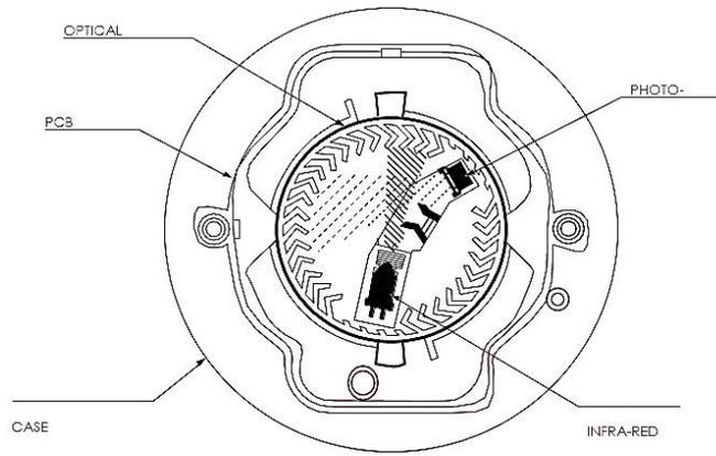
Fig.2 Top section, Series 27 Optical Smoke Detector
