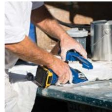
2. Remove the old pump from the sprayer.
