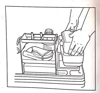
The filter bag and frame are hel in place in the housing by a rubber grommet on the franme which fits over a maetal tube.
