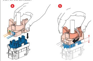
Spreading cables ensures that each pair is separated by the specified 13 mm.
