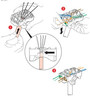
Simultaneous connection of cable strands is ensured.
