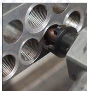
Safely re-machine gasket surfaces in seconds.
