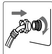
2. Connect the other end of the inlet hose to the inlet valve at the backside of the washing machine and fasten the hose tightly clockwise.
