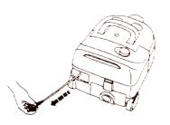
If one tries to continue to draw the cord although it is completely out (of course in an impetuous way) one may damage it.
